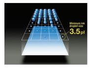
The PrecisionCore technology, as well as Variable Size Dot Technology, allow the ink droplets to be controlled to the finesse of 3.5 picolitres.
