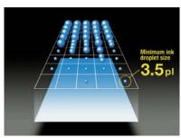
The combination of both technologies allow the ink droplets to be controlled to the finesse of 3.5 picolitres.
