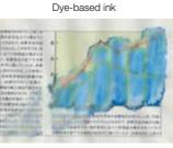
Epson pigment ink is not water soluble and firmly binds to media fibers, resisting water and other moisture. Conventional dye-based ink is water soluble so printouts can be negatively affected by water and other moisture.
