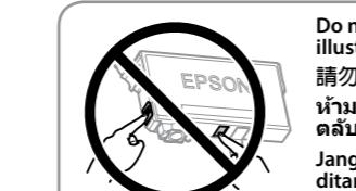
**Do not touch the sections shown in the illustration of the cartridge.**
