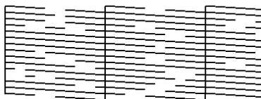
Example of clogged nozzles
