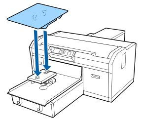
After replacing the platen with a different size, we recommend you correct print misalignment (Head Alignment).
