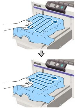
When loading a T-shirt coated with pre-treatment liquid, or when the grip pad tool gets caught due to the characteristics of the fabric, use the grip pad tool with a release sheet such as silicon paper on the T-shirt as shown in the figure.
