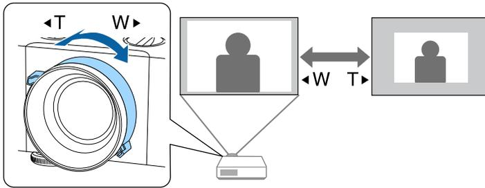
You can correct the focus using the focus ring.
