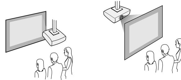
Select the correct **Projection** option in the projector's **Installation** menu according to the installation method being used. If necessary, turn on the **Inv Direction Button** setting in the projector's **Operation** menu and adjust the **Menu Rotation** setting in the projector's **Display** menu.
