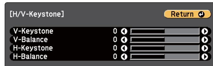
**6** Use the arrow buttons on the projector or the remote control to select between vertical and horizontal keystone correction and to adjust the image shape as necessary.
