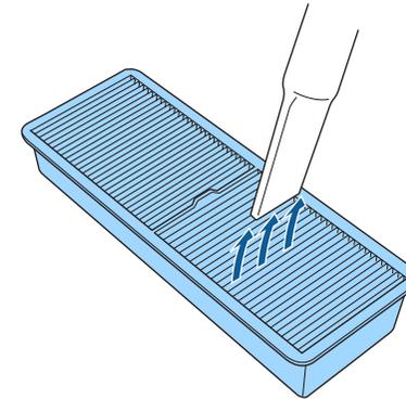
**6** Tap each side of the air filter 4 to 5 times to shake off any excess dust.
