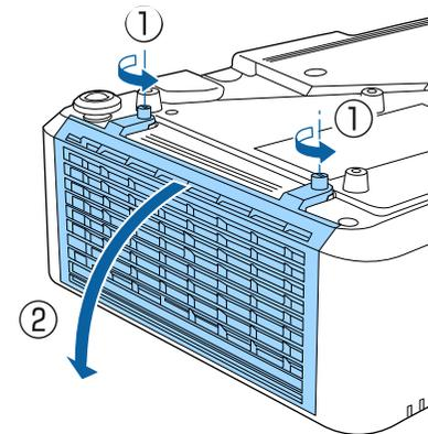
**5** Pull the air filter out of the projector.
