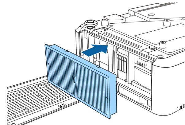
**9** Close the air filter cover and tighten the screws.
