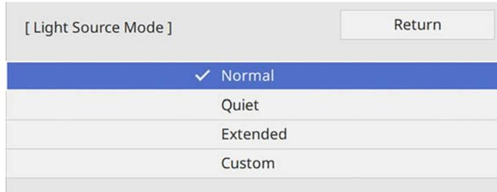
**8** If you set the **Light Source Mode** setting to **Custom**, select **Brightness Level** and use the left and right arrow buttons to select the brightness.
