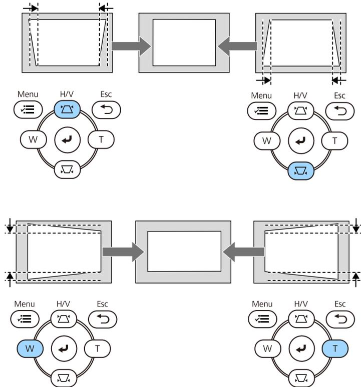
• If the projector is installed out of your reach, you can also correct the shape of the image using the remote control.
