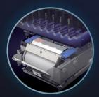
An easy-to-replace cloth wiper roll continuously wipes the printhead nozzles clean to remove fluff that can cause nozzle clogging.
