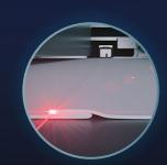
Dual head-strike sensors detect any folds or wrinkles that may cause the fabric to come into direct contact with the printheads. If folds or wrinkles are detected, the sensors immediately stop the carriage to avert a potential head strike.
