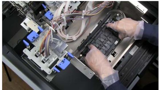
**22** Place the used Print Head that you removed on the lid of the protective case.
