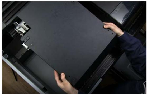
After removing the cover, place it on the top of the Printer Cover with the inside facing upward.
