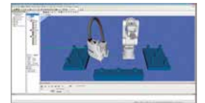
3D simulator for workcell layout and toolpath program testing
