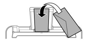
☐ Fan and align the edges of the envelopes before loading. When the stacked envelopes are puffed up with air, press them down to flatten them before loading.
