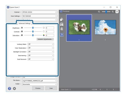
You can adjust the scanned image using detailed settings that are suitable for photos or pictures, such as the following.
