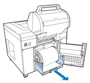
8 Remove the Spindle unit.
