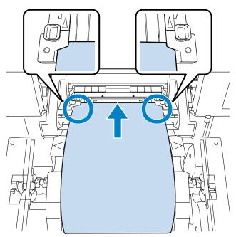
4 Insert until the leading edge appears at the position shown in the illustration below.
