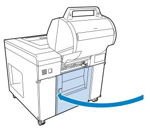
For the Dual Roll Model, press the front roll paper feeder down as far as it will go. Check that the front roll paper feeder is fixed in place.
