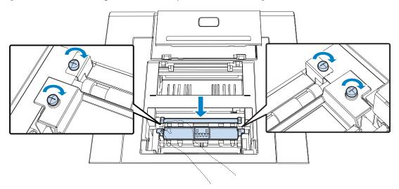
8 Push the back printing unit all the way in, and then holding the handle in the center push the unit up until it locks in place.
