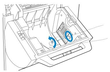
Do not remove the screw for the rear roll paper feeder. After loosening the screw, slide as shown in the following illustration.
