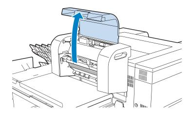
After loosening the upper cover screws by hand on the left and right, remove the upper cover.
