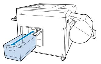
Grip the handle on the back printing unit, and pull it down and out.
