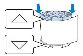
5 Place the Spindle unit on its side so that the paper is in the position shown below.
