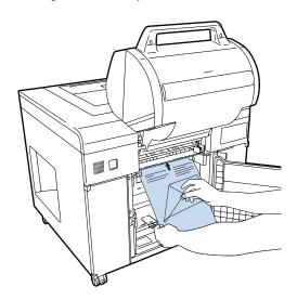
Remove the Cleaning Sheet from the rear roll paper feeder after a warning buzzer sounds indicating that cleaning is complete. Finally, install the Spindle unit for the rear roll paper feeder as it was before.
