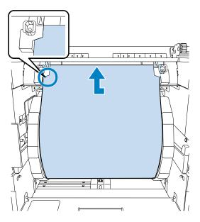
Insert until the leading edge of the paper is visible beyond the roller as shown in the illustration below.
