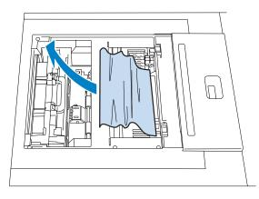
Manually move the Print Head Unit in the opposite direction to the visible paper.
