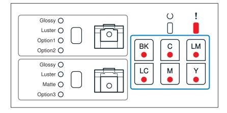
Press lightly on the expended ink cartridge (ink cartridge with the lit Ink status light), and remove the cartridge.
