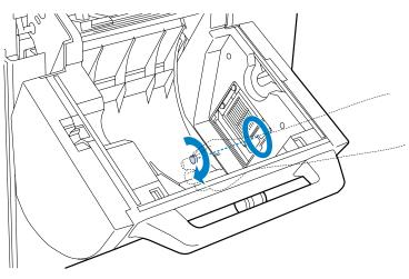
For the rear roll paper feeder, after sliding the screw, turn it by hand to fix it in place.
