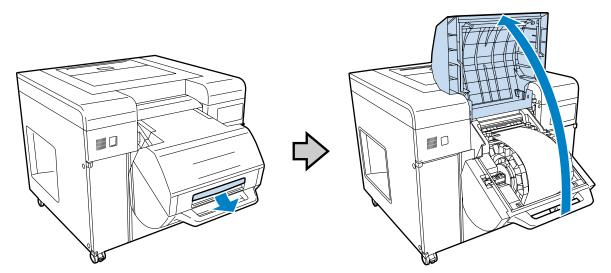
A Remove the paper from the Paper feed slot, and rewind the paper.
