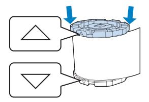
Place the Spindle unit on its side so that the paper is in the position shown below.
