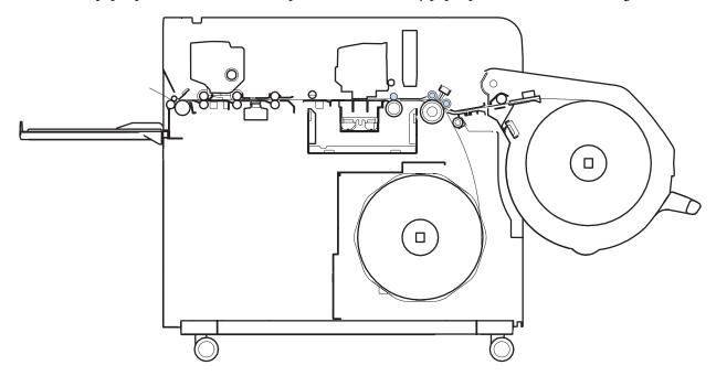
After removing the Spindle unit from the rear roll paper feeder and inserting the Cleaning Sheet into the Paper feed slot, peel off the adhesive tape. Slide the bottom edge of the Cleaning Sheet into the printer, and then close the rear roll cover. For the Single Roll Model, cleaning starts at this point. For the Dual Roll Model, push down the front roll paper feeder to its former position to start cleaning automatically.
