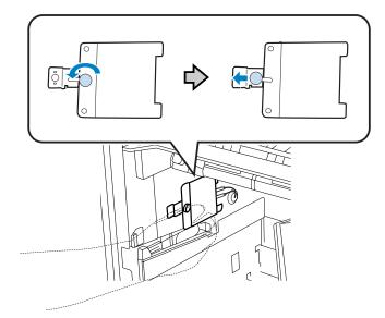
Slowly remove the humidity control unit in the direction shown by the arrow.
