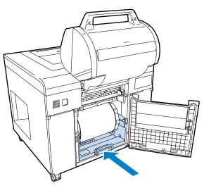
Adjust the position of the paper width guides to the width of the paper.
