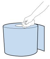
Set the Flange on the paper surface from which paper particles have been wiped away.
