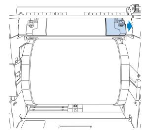
5 Match the left edge of the paper with the left Paper width guide, and pass the leading edge of the paper through the groove in the paper width guides.
